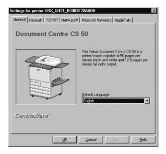
The **Network** tab is used to modify printer network settings such as Network Type, Frame Type, and Connection Type. The **TCP/IP**, **NetWare**, **Microsoft Networks**, and **AppleTalk** tabs are used to modify printer settings that are specific to those network environments.
